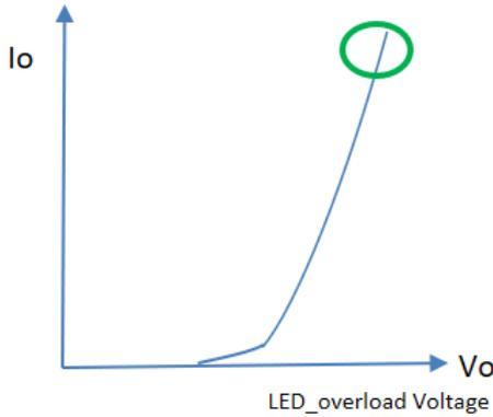
Set  $V_{\text{overload}}$  close to, but higher than the maximum forward voltage for optimized performance. The greater the difference between the  $V_{\text{overload}}$  setting and the maximum forward voltage, the higher the overload stress will be. The  $V_{\text{overload}}$  setting must be higher than  $V_f$ .
